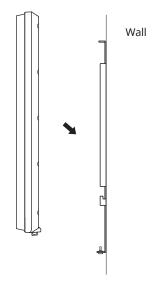
**4** Connect FaceStation F2 to the bracket by rotating the product fixing screw of FaceStation F2.
