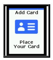
Place the card to register on the LCD. To cancel and exit the registration, press [ESC] button.
