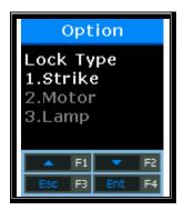
Set to '1' when the terminal is connected to the strike type or automatic door, and '2' when it is connected to the motor lock.
