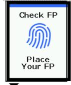
Place your finger on the fingerprint sensor, and the red light is on the fingerprint input window. Keep your finger until the red light is off with a beep sound.
